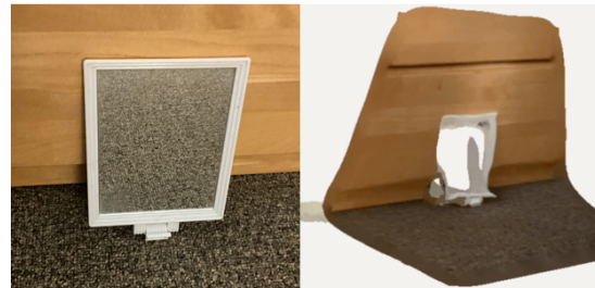
Fig. 1. Mirror Reconstruction with Conventional LiDAR. Conventional LiDAR systems fail to map the 3D shape of mirrors because mirrors reflect light away from the sensor. As a result, holes appear in the reconstruction.
