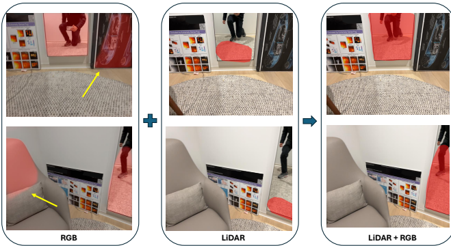
Fig. 12. Refining RGB Segmentation with LiDAR. LiDAR corrects the incorrect mirror mask from RGB segmentation. First column shows the incorrect mirror mask detected by RGB-based segmentator (MirrorNet), indicated by the yellow arrows. Second column shows masks from LiDAR mirror detection (mesh reconstruction from the detected points). Third column shows the combined mirror masks from both sensors. RGB gives a denser detection, while LiDAR can identifies the true mirror segment.
