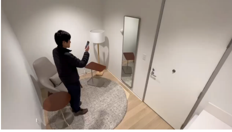
Fig. 5. Experimental Setup. We use a handheld device for 3D room scanning, eliminating the need for complex research-grade equipment or manual calibration.
